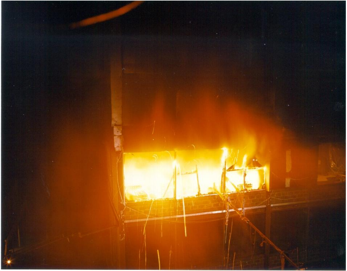
Photograph 4 BRE Corner fire test
