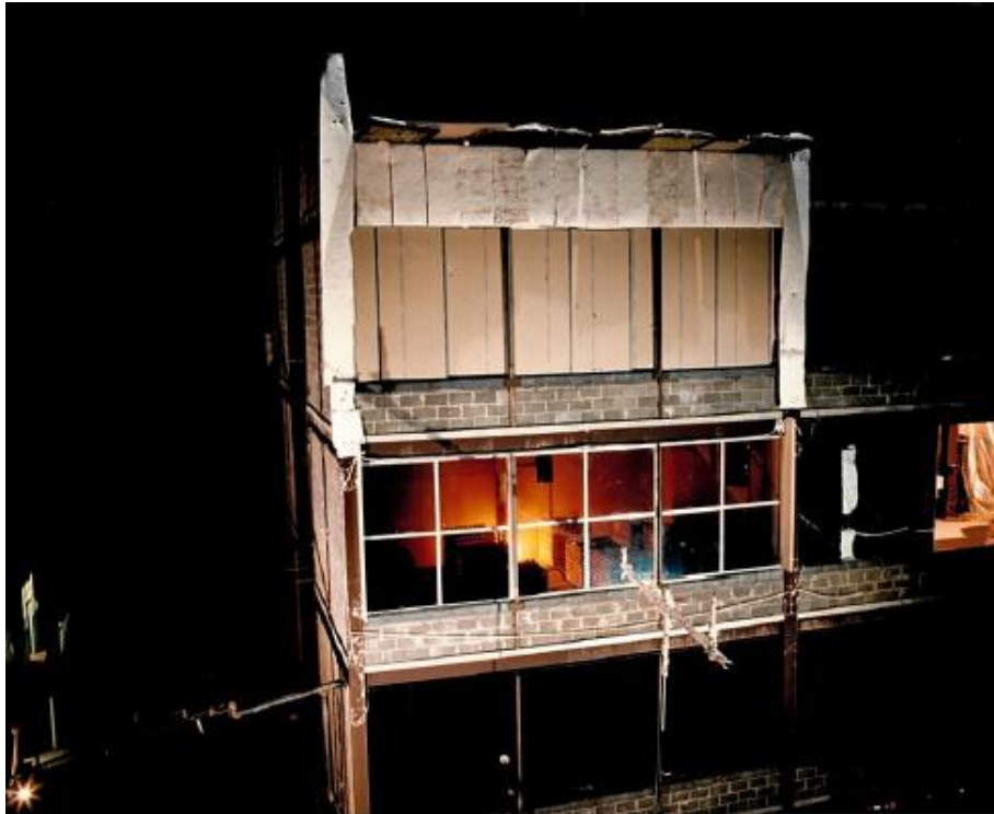
Photograph 3 Corner fire test prior to ignition – view from outside
