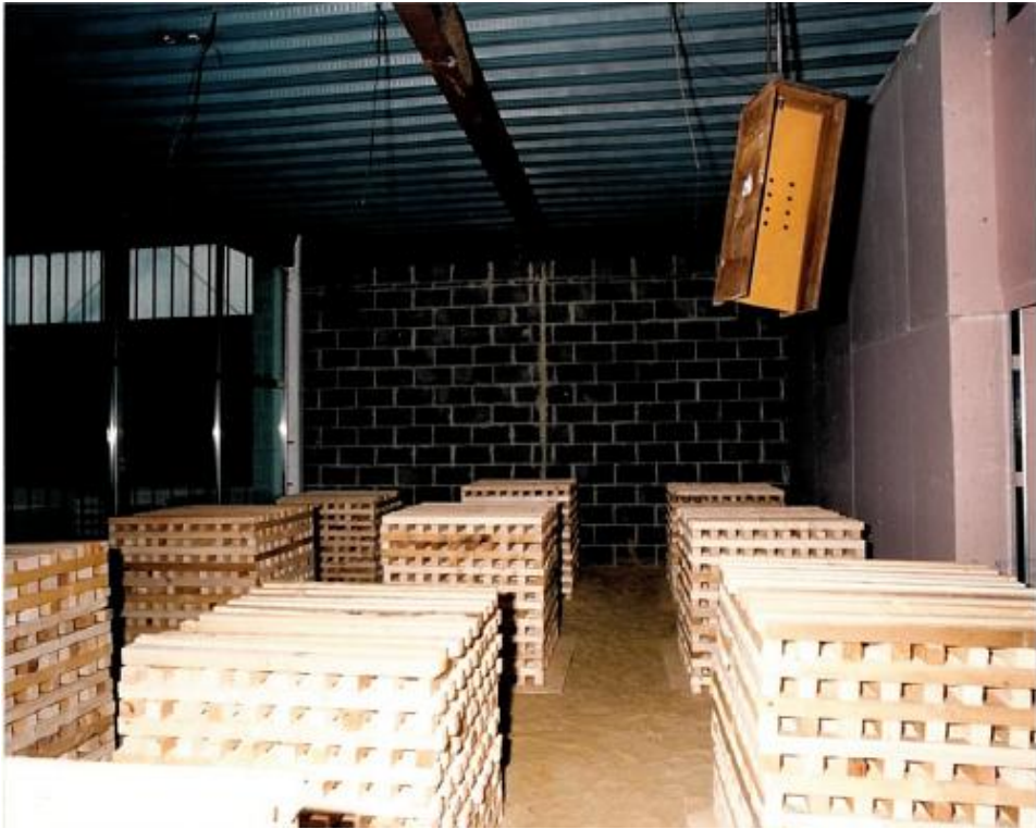
Photograph 2 Corner fire test prior to ignition – view from inside
