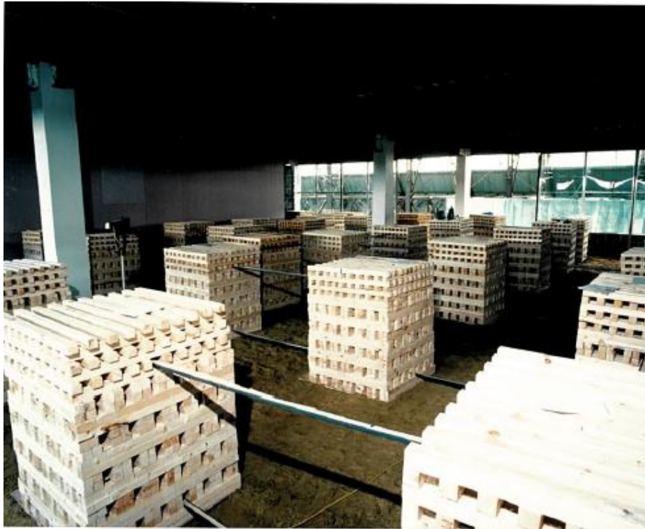
Photograph 6 Large compartment fire test prior to ignition showing crib layout
