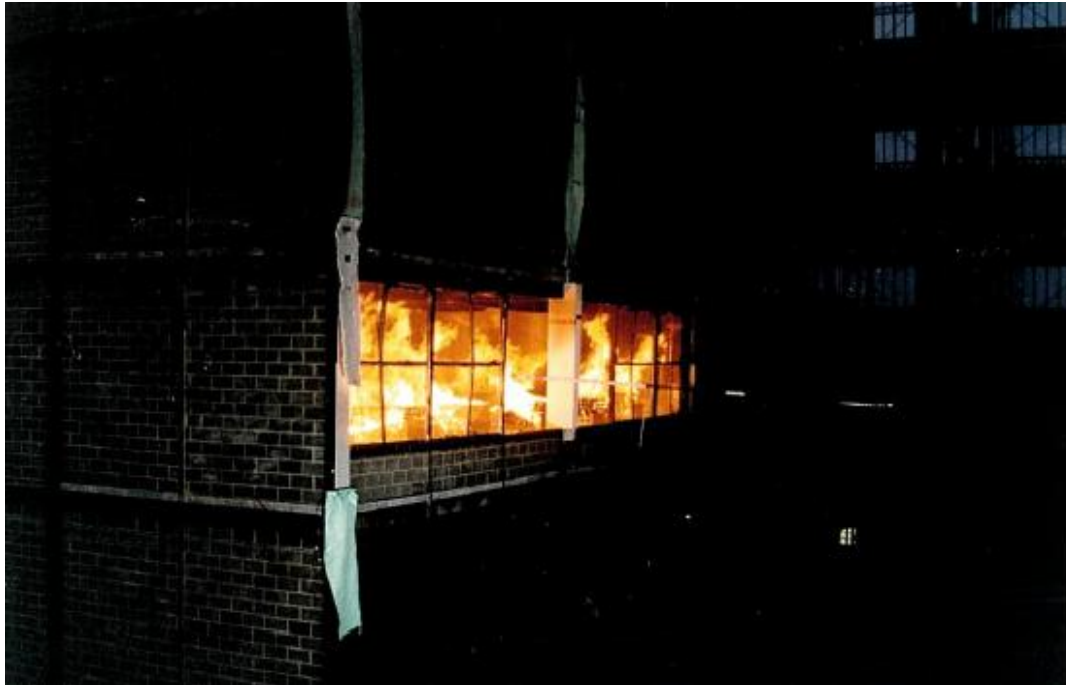
Photograph 7 Post-flashover fire development – cribs burning individually
